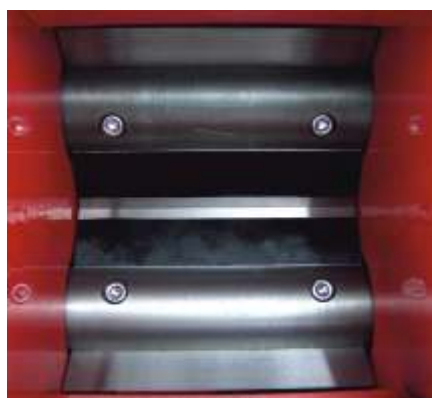
The gap between the blades is c. 0,1 mm. Which means the logger can process even very small branches.
